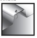
FOR PROPER APPLICATION, THE USE OF IMPACT DRIVERS ARE NOT RECOMMENDED FOR POWDER COATED OR ANY WET PAINTED FASTENER
