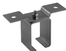
BC3-301S - 103010300 Ceiling bracket Includes mounting flange for BC301 track Packaged with (2) lag bolts to fasten to header
