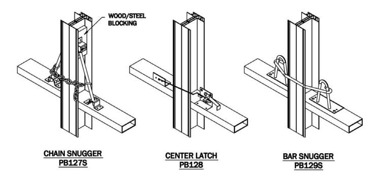
1 INSTALL A LATCH AT THE JAMB. A CHAIN SNUGGER, JAMB LATCH OR A JAMB STOP ARE THE BEST OPTIONS. THE MOST POPULAR WAY TO INSTALL EACH IS SHOWN BELOW.
